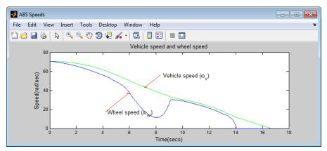
By comparing these plots with the plots in "Lesson 1: Run the Time-Based Model" on page 2-30, you can see that the delay introduced between the ABS controller and the braking system significantly degrades the performance of the braking system:
