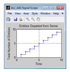
After an entity departs from the Single Server block, the block updates its output signal at the #d port. The updated values are reflected in the plot and highlighted with plotting markers. From the plot, you can make these observations:
