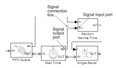
In a discrete-event system, the signal input port coming into a block changes to an empty arrow when you perform update diagram:
