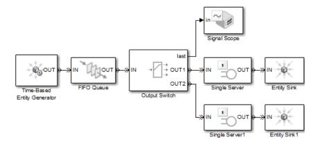
This deterministic model creates one entity every second and attempts to advance the entity to one of two servers. The two servers have different service times, both greater than 1 second. The server with the longer service time becomes available less frequently and has a smaller throughput. The FIFO Queue block stores entities while both servers are busy. After any server becomes available, an entity in the queue advances to the Output Switch, which outputs that entity to that server.
