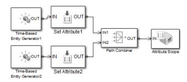
• **Merging queues:** Multiple queues merge into a single queue. (You might also use an Input Switch block for this, depending on the desired sequencing of entities in the single queue.)
