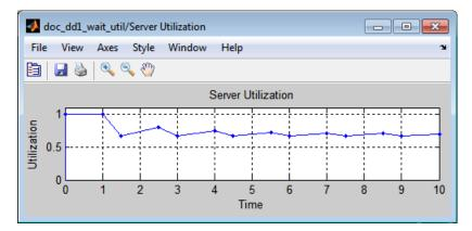
• The average waiting time in the queue increases throughout the simulation if the intergeneration time is small (such as 0.3) because the queue gets longer and longer.
