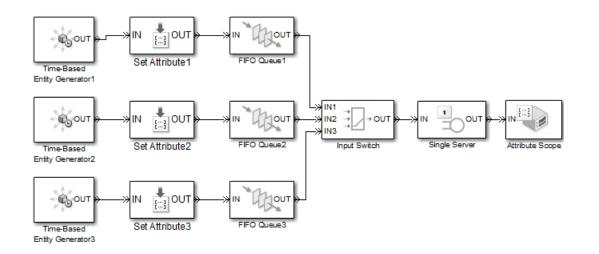
Consider the following example, in which three sets of entities attempt to arrive at an Input Switch block with the round-robin switching criterion.
