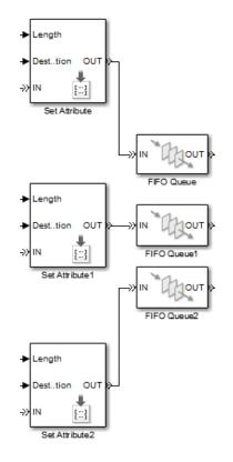
The queue uses a FIFO queuing discipline, which does not take into account the destination of each packet. Note that such a model can suffer from "head-of-queue blocking," which occurs when a packet *not* at the head of the queue is forced to wait even when its destination is available, just because the packet at the head of the queue is aiming for an unavailable destination.
